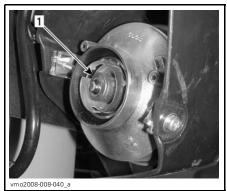
PULL ON BULB TO REMOVE THEN REPLACE BULB 1. Bulb
